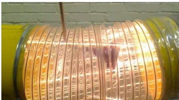
Figure 3. Tracks of hot metal droplets at the entry of the cyclone
